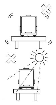
C. The best settlement site should be in a sheltered corner, on the stable marble platform and far away from door, window, radiator and the air outlet of the air conditioning equipment.
